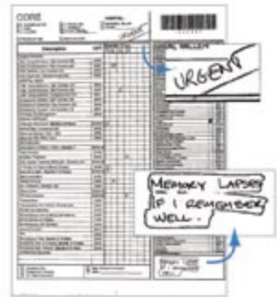
VRS Scanning: VRS easily handles both the light and dark text in this document. It suppresses the shading for easier recognition of the check marks, and makes the highlighted text clearly visible. This image is as clear as it can be for the automated capture of information, and the file size has been reduced to an optimal 65 Kbytes.
