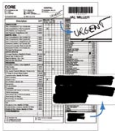
Conventional Scanning Without VRS: Scanning the same form in black-and-white (bitonal) makes the pencil text easier to read and reduces the file size to 88 Kbytes. But the highlighted text is completely lost, and the shaded boxes become shades of gray, which would confuse a system that is looking for the check marks.
